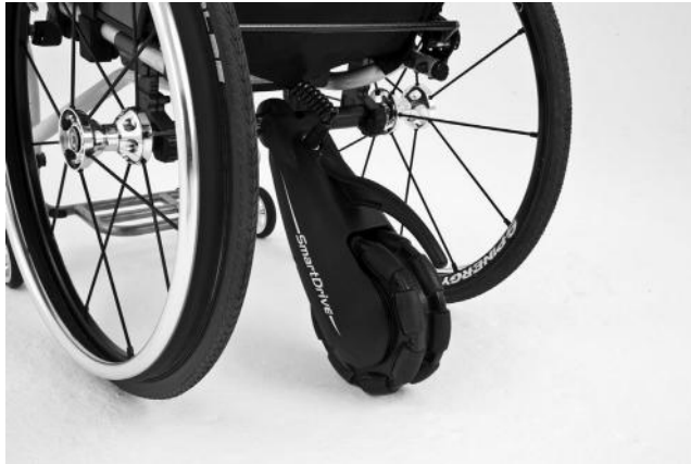
FIGURE 24.1 SmartDrive installed on a user's wheelchair.
